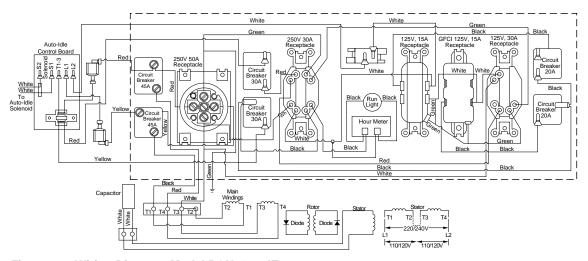
Figure 23 - Wiring Diagram, Model PGH11000IE
